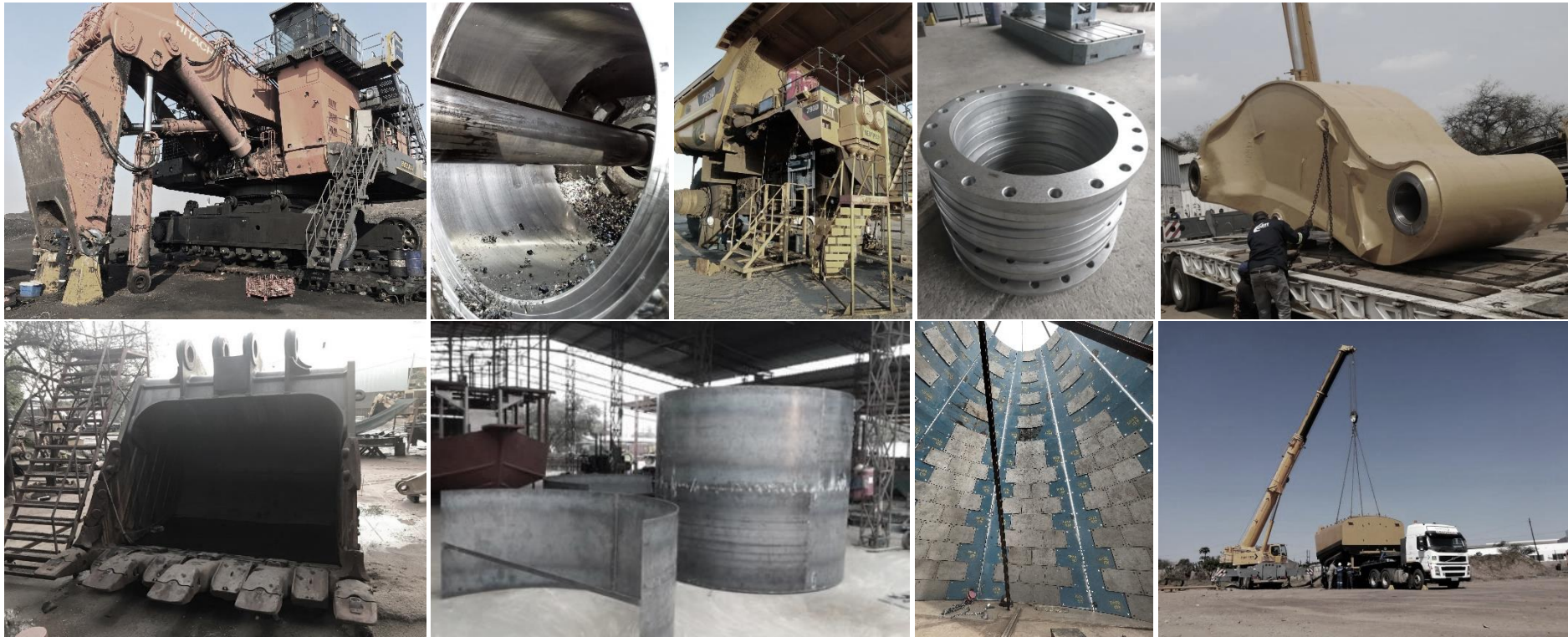
1. Line-boring of a Hitachi EX8000 sitch 2. Heavy-duty line-boring 3. Portable milling of a strut-face for a Caterpillar 793D mining truck 4. Fabrication of machined flanges 5. Refurbishment of a Caterpillar bucket holding arm 6. Reinforcement and re-lining of heavy-duty excavator buckets 7. Pipping and boiler-making fabrication 8. Fabrication of a 500T Silo cone 9. Refurbishment of a Caterpillar water-carrying vessel
